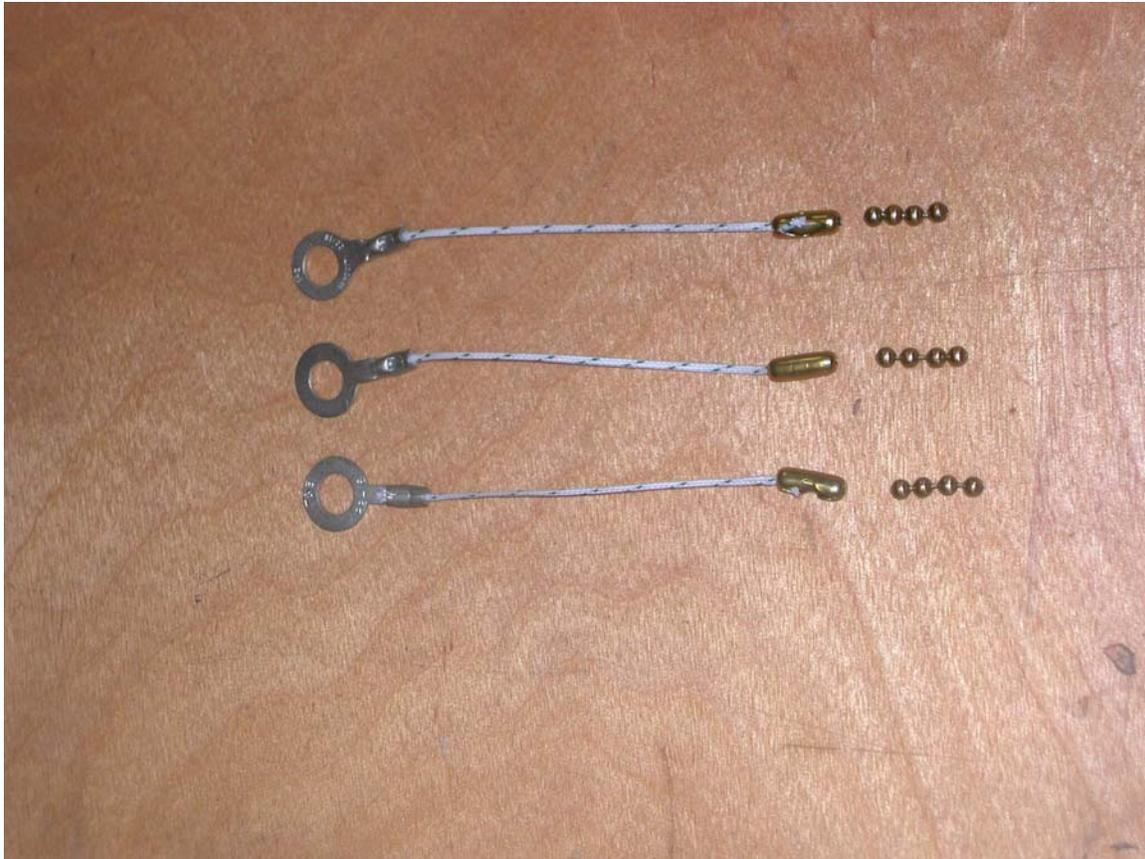
Then, I assembled the brass stud, brass nuts and guy ring sections into the special IEC. The nuts are threaded onto the stud, with the three rings in between them. The nuts are spaced apart so that the rings can rotate freely, but not so far that there is only a short section of stud to attach the HFp element. On mine, there was about 5/8" of stud on the outside of each nut, and the space between the nuts was about 3/8". I used Loctite 262 thread locker to hold the nuts in place.
