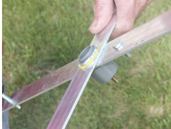
Figure 1: Installed Center Insulator
