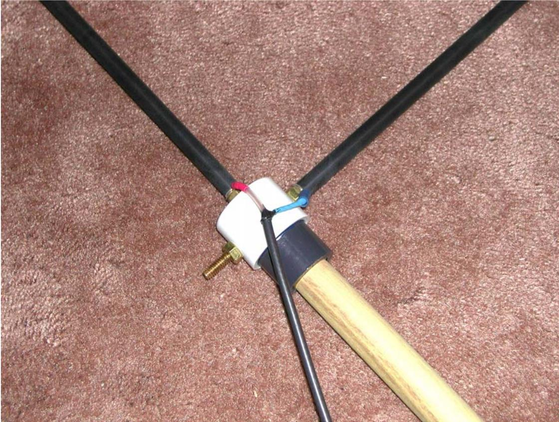
The HFp Dipole set up as an “L” antenna
