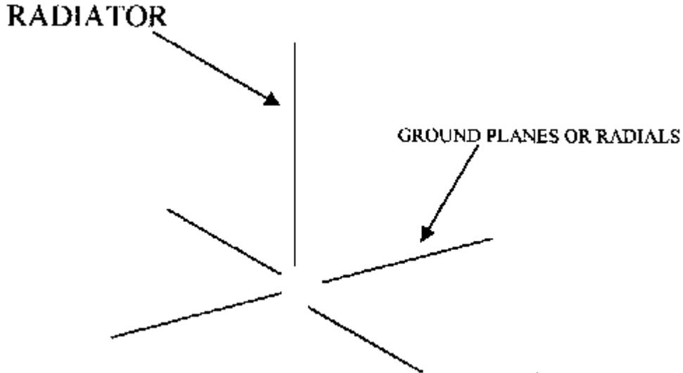
If the radials on a ground-plane antenna are bent down to about a 45 degree angle, the impedance rises to about 50 Ohms. This makes a very good match to 50 Ohm coax.
